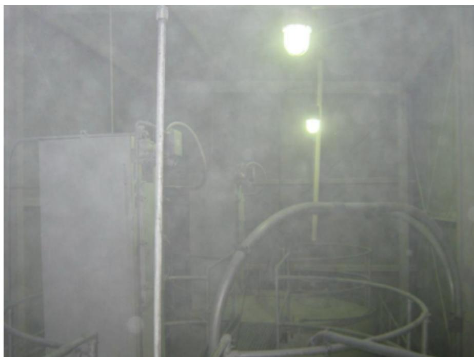
Leaving aside the fact that it may be toxic to breathe, the dust fouling the air in this space may be combustible, i.e., apt to catch fire and explode. If it **is**, in fact, combustible, heat from the machinery and lighting fixtures might be the ignition source that causes it to go off.
