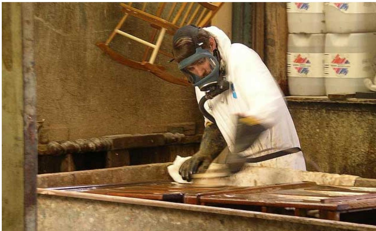
The worker in this picture (which, ironically enough comes from OSHA's own Safe Workplaces photo contest) is using appropriate hand protection and a full face respirator mask. But while he's wearing coverall body protection his hood is hanging limply around his shoulders instead of covering his head.
