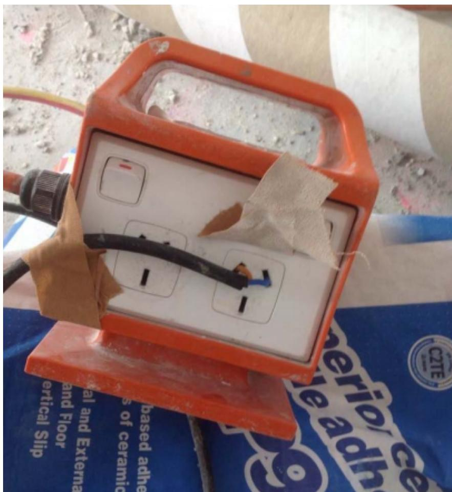
Making do with what you have is good advice in many situations, but in the world of workplace safety, making do often translates into taking unsafe shortcuts. Here we have a situation where someone has shoved bare electrical wires into an electrical outlet and then taped the makeshift wiring to hold it in place. Hopefully necessity won't become the mother of electrocution. (WorkSafeVictoria, Australia)
