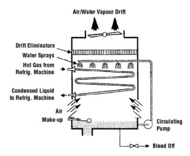
Cooling towers and evaporative condensers may contain Legionella and other microorganisms brought in by circulating air or water.
