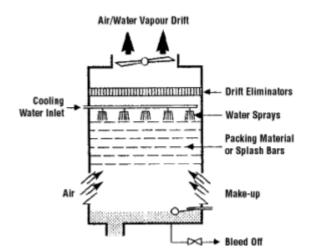
While falling through the tower, some of the water evaporates. Because evaporation consumes heat, the remaining water is cooled. Air pushed through the tower by fans also cools the water. Some droplets, known as drift, are carried out of the tower by the air stream produced by the fans. This water loss is reduced by a drift eliminator positioned at the top of the tower. The cool water collects at the bottom of the tower and is pumped back for another cycle.
