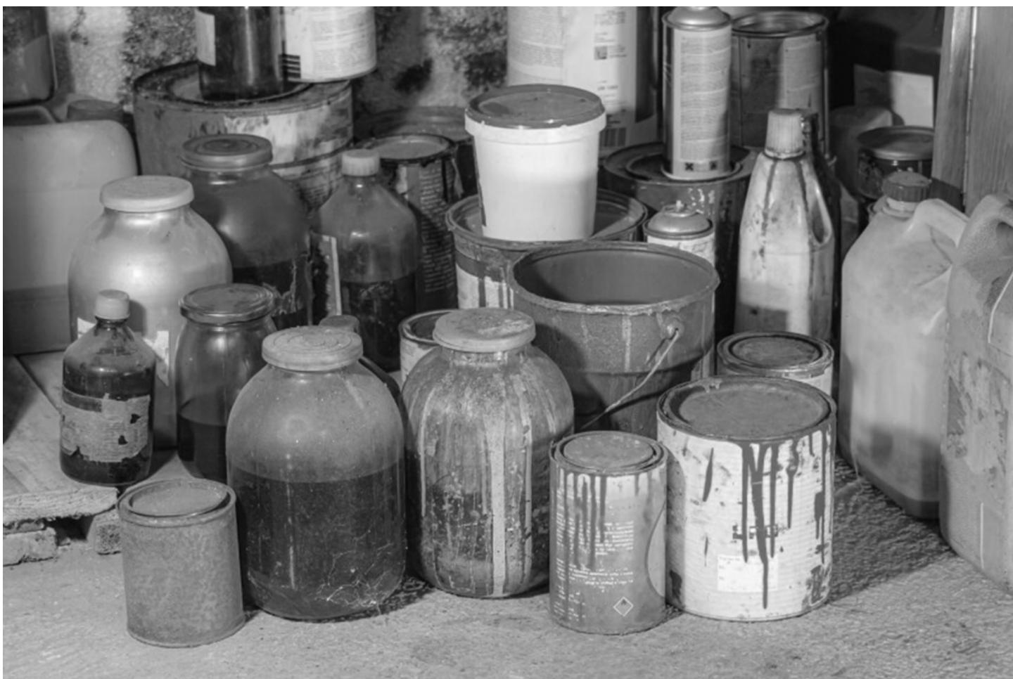
This image reveals a highly disorganized collection of chemical containers, many of which are unlabeled, rusted, or leaking. Such poor practices significantly increase the risk of chemical exposure, fire, poisoning, or improper disposal. In workplaces and storage areas, all chemical containers must be clearly labeled with the substance name, hazard symbols, and safety instructions to comply with WHMIS (in Canada) or OSHA HazCom (in the U.S.).
