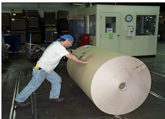
These paper rolls weigh about 3,000 pounds. Just imagine how much stress it puts on the worker's back, shoulders, arms and wrists to roll these monsters by hand—especially across a concrete, sloped floor that's pocked with holes and latticed with roll stand tracks! It's a musculoskeletal disorder (MSD) just waiting to happen.
