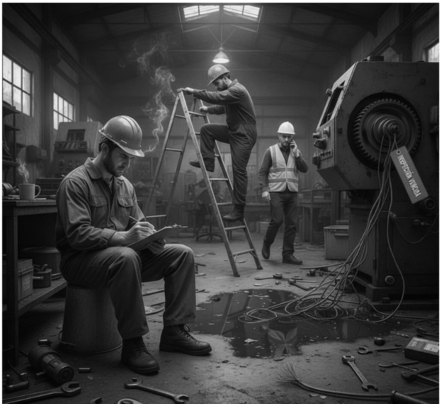
This image highlights a hazardous work environment full of common yet serious inspection failures. Tools are scattered across the floor, creating trip hazards. A large puddle of liquid poses a slip risk. A lockout tag is visible but the area remains cluttered and potentially energized. A worker is climbing a ladder
