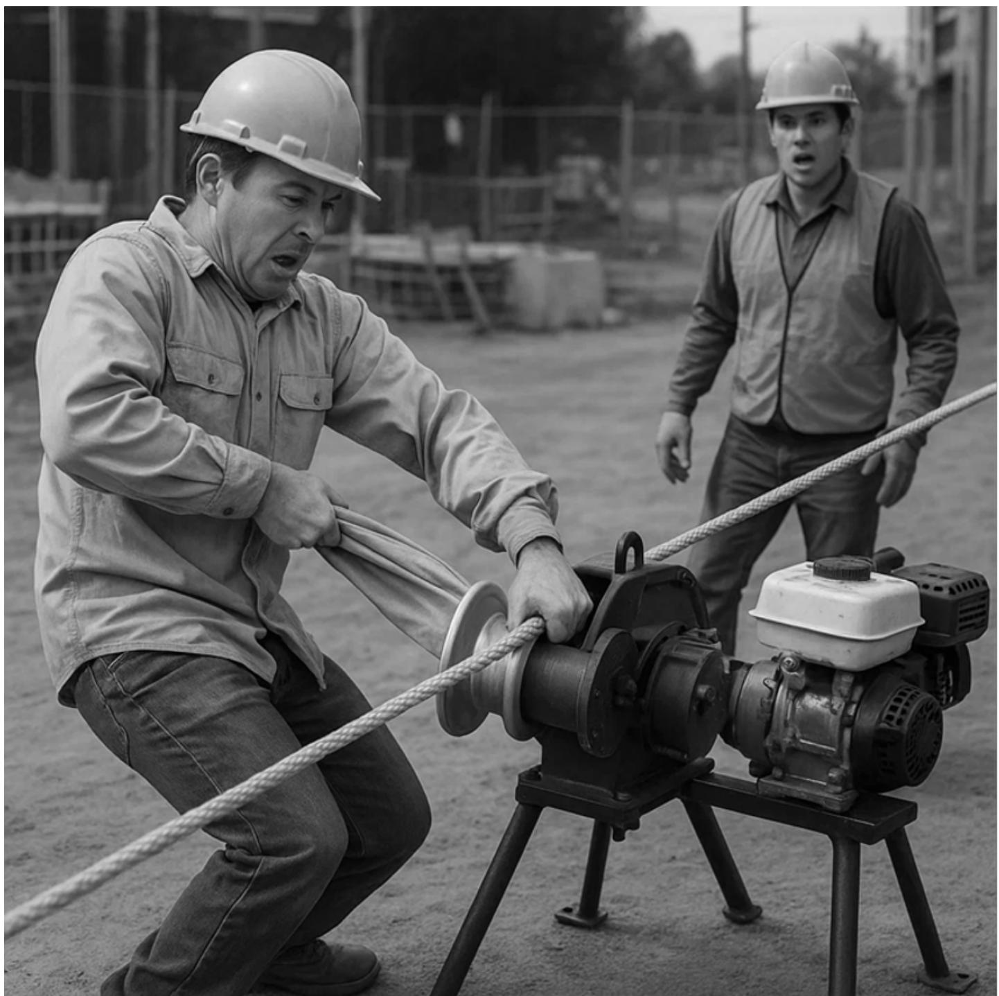
The worker is dangerously close to a spinning capstan hoist drum and is pulling the rope by hand without proper guarding, standoff tools, or protective spacing. This exposes them to severe entanglement and crush hazards. The lack of distance and improper handling technique can result in fingers, hands, or clothing being pulled into the rotating mechanism. Additionally, the worker nearby appears alarmed but is not intervening or reporting the incident.
