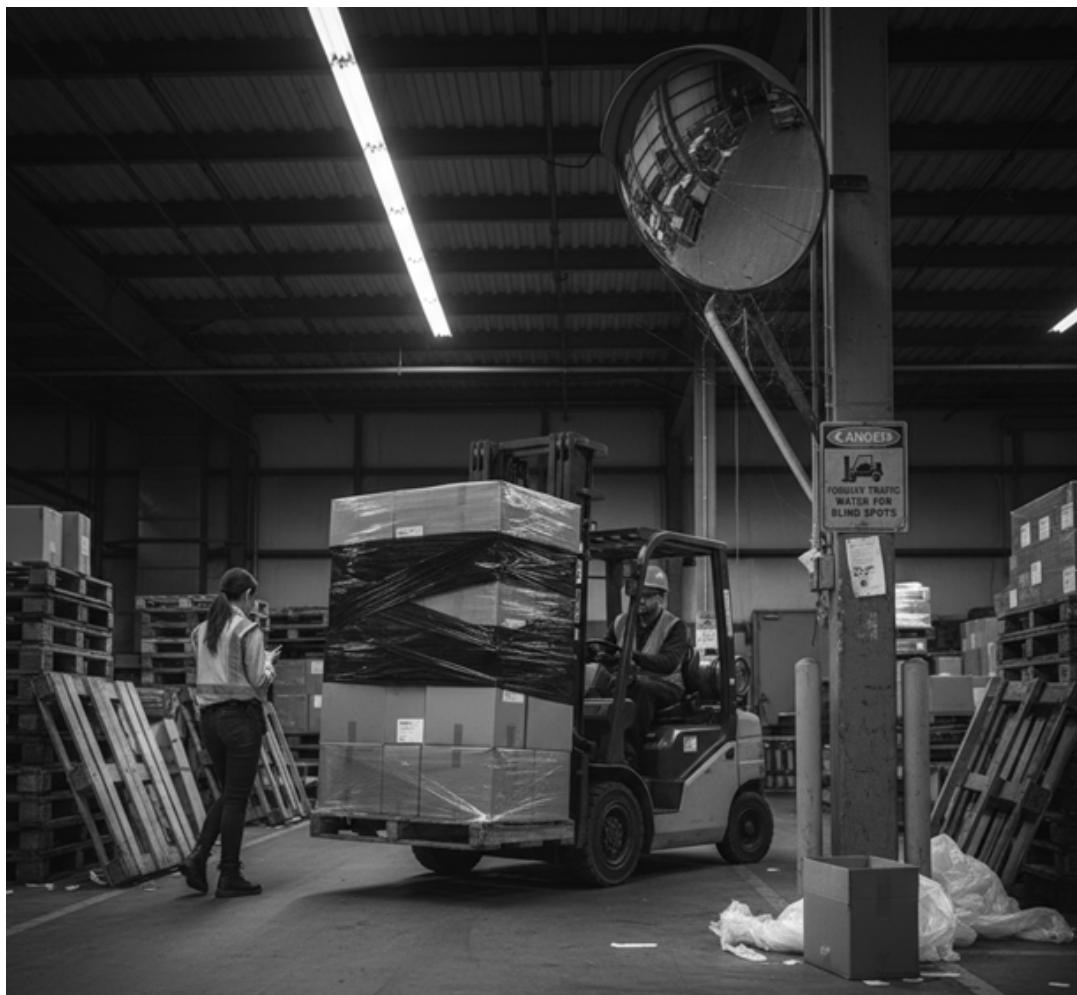
The forklift operator's forward view is completely blocked by an oversized load, and a pedestrian is walking directly into the forklift's blind spot without establishing eye contact or ensuring the operator sees her. Despite the presence of a convex mirror and a warning sign, the layout and behavior create a high risk of a struck-by incident.
