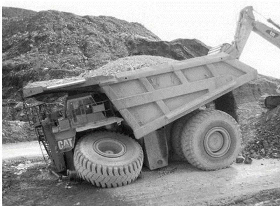
**What's wrong in this picture?** Dump truck could not resist overloading! "A raised truck bed can easily overturn due to its size and weight," states MSHA. "Uneven ground, unbalanced load, and/or underinflated work tires increase the hazards associated with this task. These hazards can be avoided with proper training and implementation of best practices."
